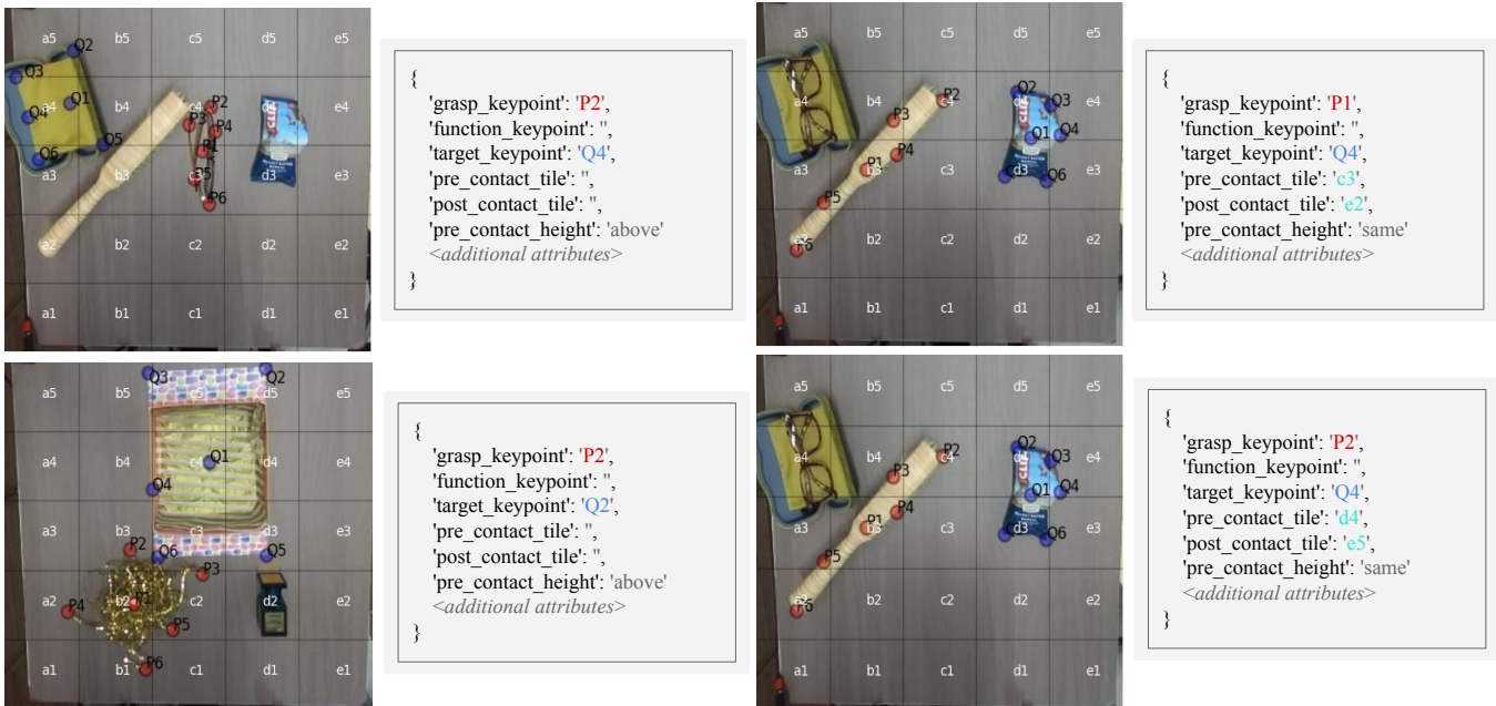
Fig. 8: Qualitative results of ablation studies. Without keypoint description or chain-of-thought prompting, the model can make mistakes in keypoint prediction (left column) and waypoint prediction (right column).
